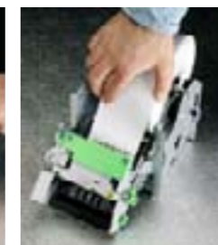
Easy Paper Load – simply "lift and tilt" mechanism and insert paper
